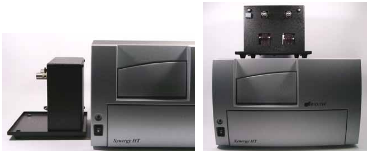
Figures 10 and 11: Possible locations for the dispense module, to the left or on top of the instrument.
