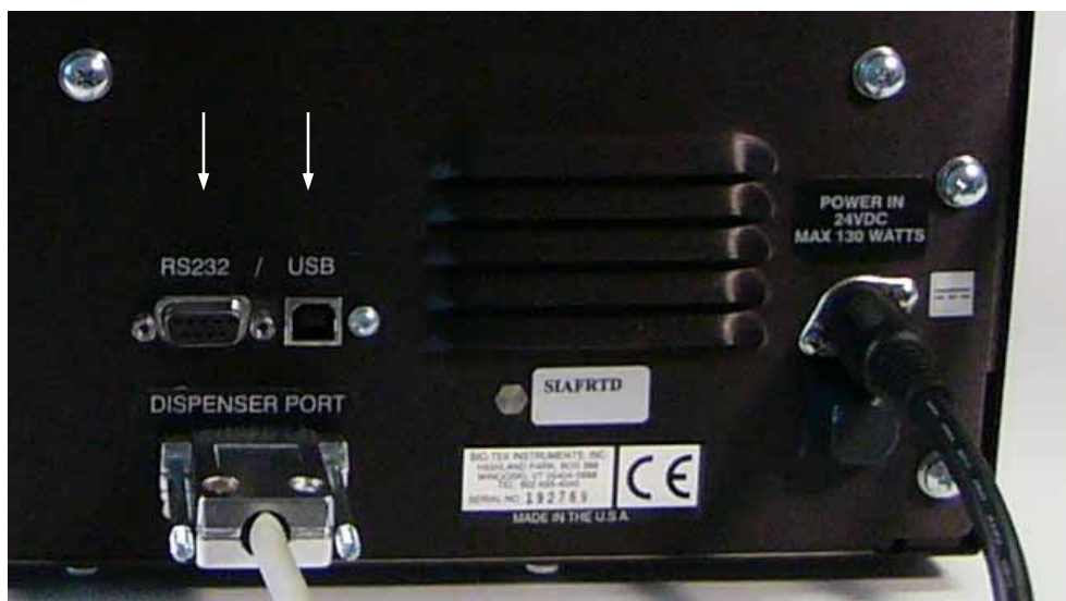
Figure 15: RS-232 serial and USB ports on the rear panel (injector model shown)
