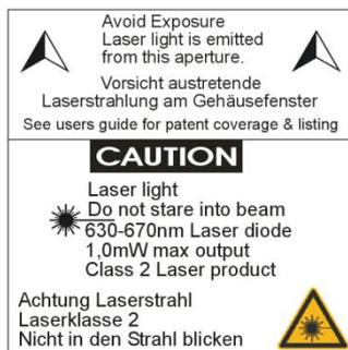
Figure 1: Warning Label on barcode Reader
