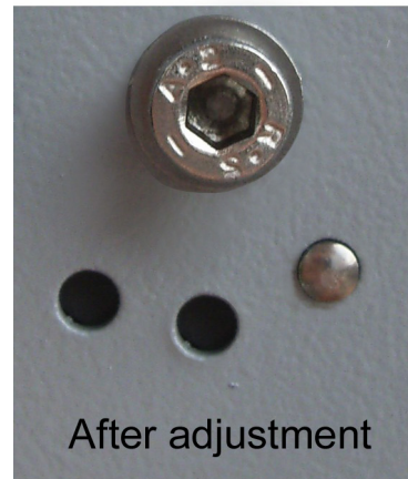
Figure 12: Stacker II bottom view. If "X2" is out of range: Move all holders counter-clockwise (right) so the pin will fit into the right hole.
