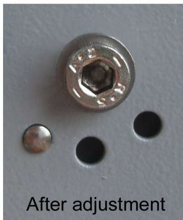
Figure 11: Stacker II bottom view. If "X1" is out of range: Move all holders clockwise (left) so the pin will fit into the left hole.
