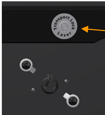
Fig. 3: Top view of the laser transport lock screw in the reagent box
