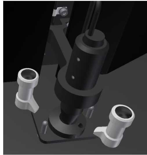
Figure 8: Quick-fix - pull up and turn to change injection head
